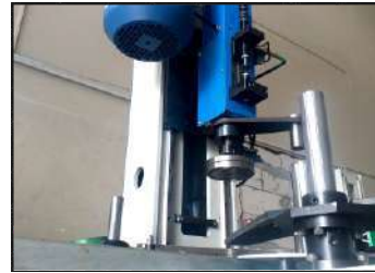
Hidroprömatik Kalıp Tahrik Sistemi / Hydropneumatic mold drive system
